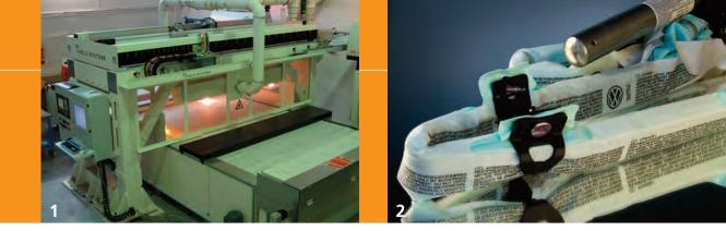
Based on many years of experience in remote processes, the Fraunhofer IWS together with HELD Systems has developed a workable industry concept. The contiLAS system realizes a processing "on the fly" in two dimensions. The remote technology allows the implementation of a laser cutting process on any cutting contours and material widths. One or several scanners can work on the fabric webs. Thus, material handling speeds of up to 25 meters per minute are achieved.
